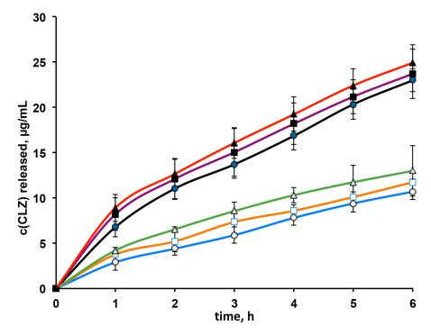
**Figure 5.** Release profiles of clonazepam (CLZ) from G1 ( $\bullet$ ), G3 ( $\blacksquare$ ) and G5 ( $\blacktriangle$ ) gel formulations and from the corresponding ones without RAMEB (white symbols).
