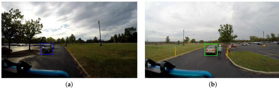
Figure 14. Examples of car detection in the GoPro video: (a) Acura SUV and (b) Toyota Corolla detected in two different frames.
