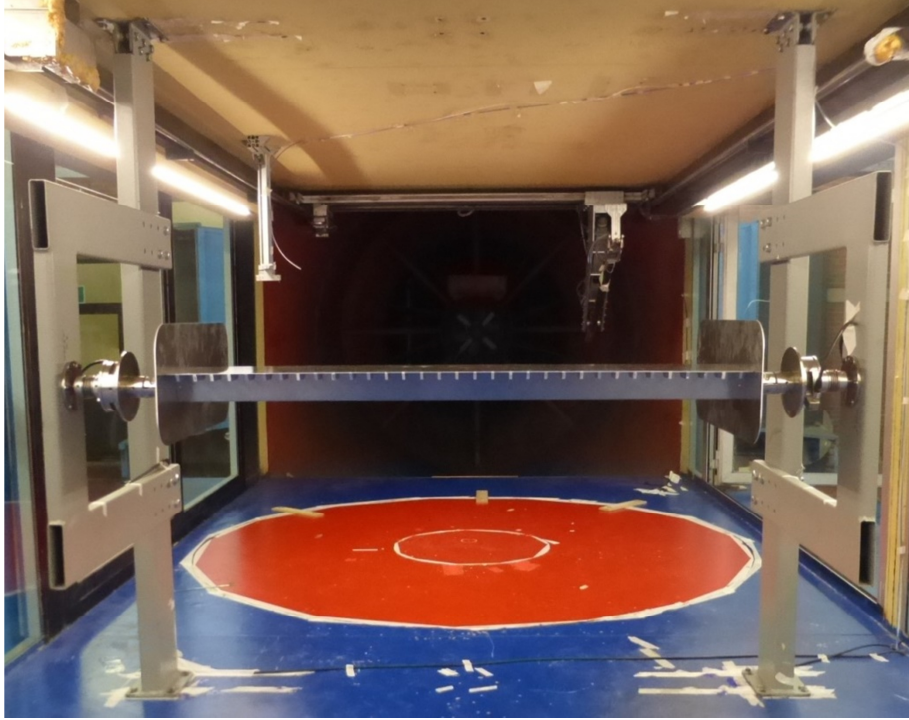
Figure 3.4. Static wind tunnel setup with manual rotation system, used for the first set of force measurements on the sectional model
