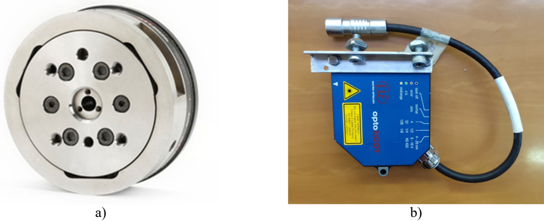
Figure 3.3. High frequency force balance (a) and laser transducer (b) used, respectively, for static and dynamic tests.
