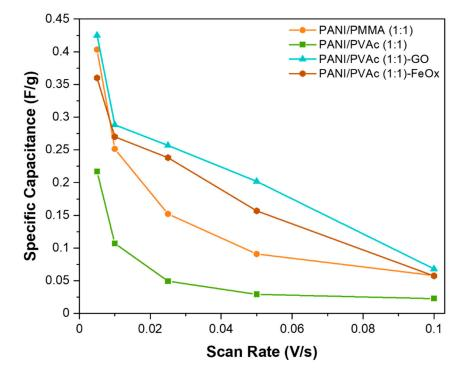
Figure 5. Specific capacitances of electrospun blended mats.
