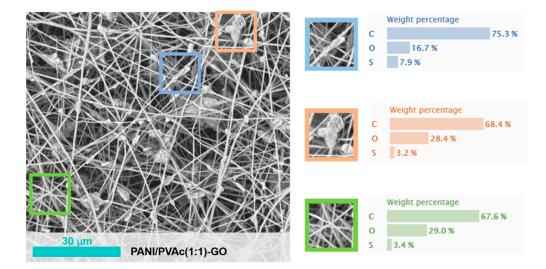
Figure 7. SEM images of PANI/PVAc (1:1)-GO and delimited EDX profiles.
