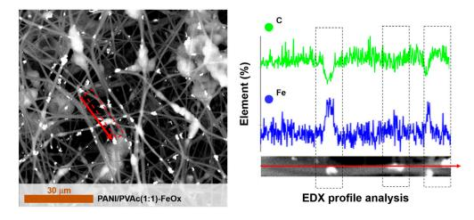
Figure 8. SEM images of PANI/PVAc (1:1)-FeO<sub>x</sub> and delimited EDX profiles.
