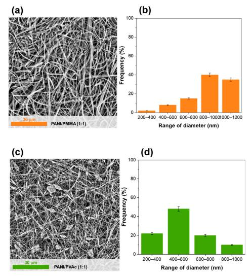
**Figure 1.** SEM images of (**a**,**b**) PANI/PMMA(1:1) nanofibers and distribution of dimensions and (**c**,**d**) PANI/PVAc (1:1) nanofibers and distribution of dimensions.
