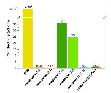
Figure 4. Electrical conductivity of as-electrospun mats.
