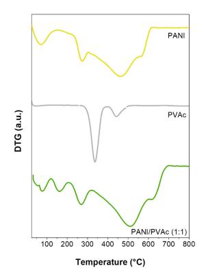
Figure 3. DTG profiles of different electrospun mats: PANI, PVAc and PANI/PVAc (1:1).
