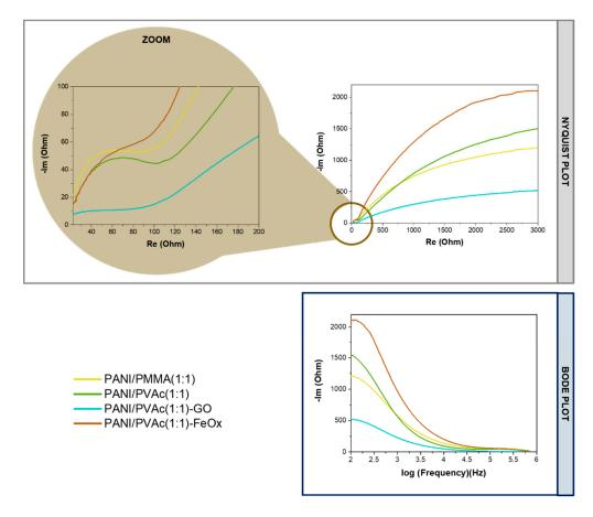
Figure 6. Impedance spectra of electrospun blended mats: Nyquist and Bode plot.
