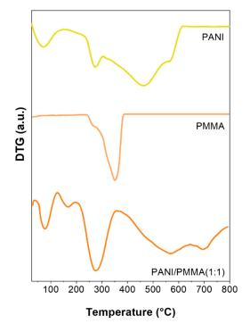
Figure 2. DTG profiles of different electrospun mats: PANI, PMMA and PANI/PMMA (1:1).
