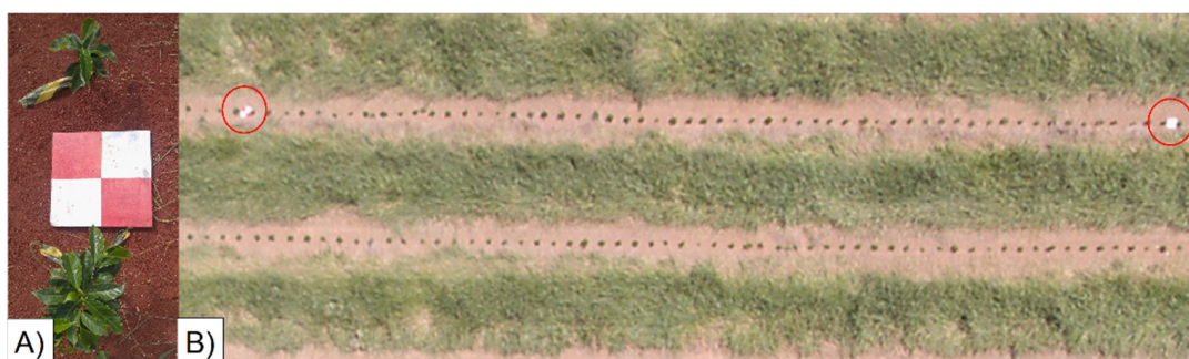
Figure 6. Control points: (A) target details, (B) targets set in the coffee tree area.
