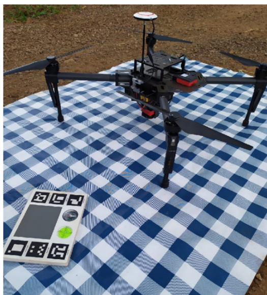
Figure 5. RPA Matrice 100 and Parrot Sequoia embedded sensor.
