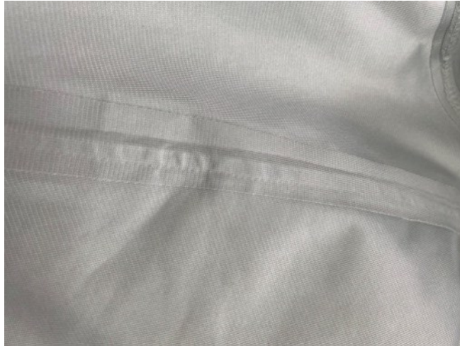
Figure 3-15: Detail of the taped seams
