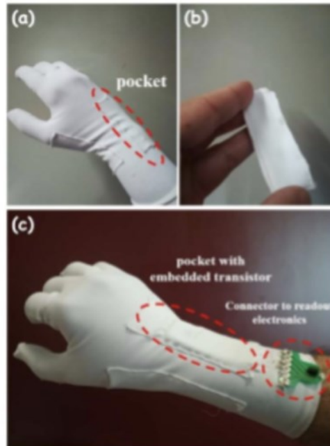
Figure 3-2: Pictures of the sensing glove: (a) the glove without sensors, where the position of the pocket is highlighted; (b) the Lycra® pouch where the OFET sensor is inserted; (c) glove provided with sensor (inserted in the pocket) and connector.
