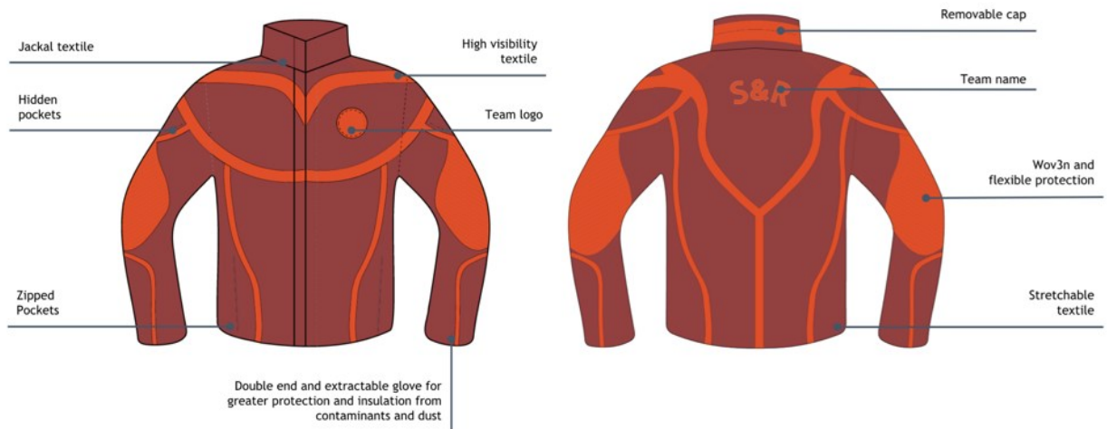
Figure 4-1: Jacket front and back views with some detail's indications
