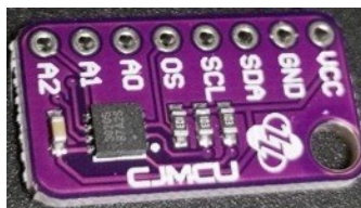
Figure 10-6: Body temperature sensor
