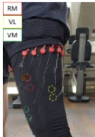
Figure 4-9: The leg sleeve fabricated for the validation of the electrodes. Three couples of PEDOT:PSS electrodes have been placed on the Vastus Medialis (VM), the Vastus Lateralis (VL), and the Rectus Femoralis (RF)
