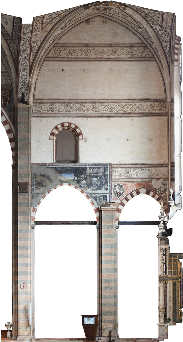
Fig. 3. Section of the transept towards the Pisanello's fresco, photogrammetric reconstruction (G. Verdiani, 2021).
