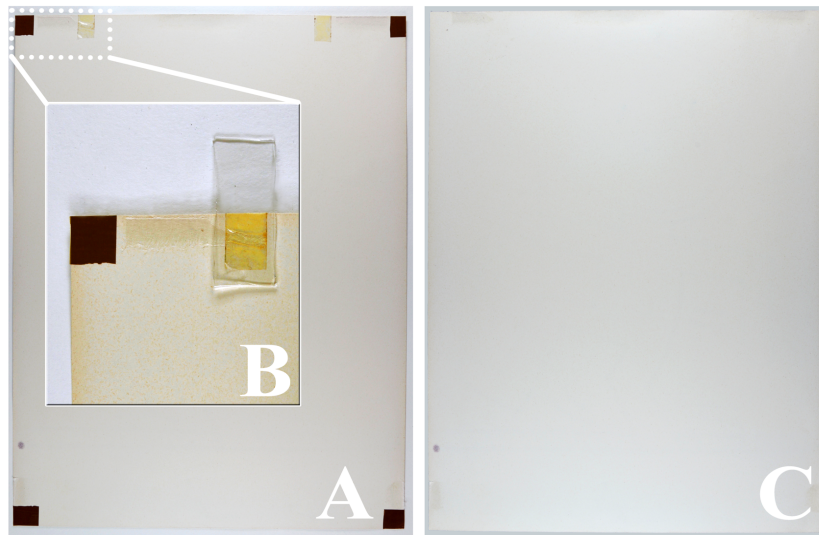
Figure 11 – (A) verso -side of the artwork by K. Haring before restoration showing the presence of the PSTs; (B) detail showing the application of a PEMA-DEC organogel; (C) verso -side of the artwork after removal of the PSTs.
