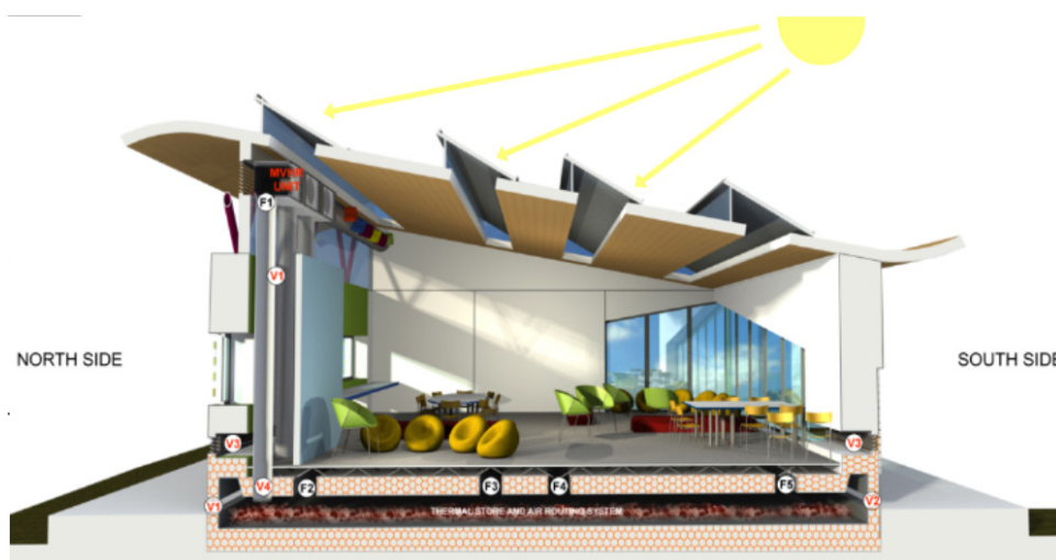
Fig.41 - Concept progettuale dell'unità scolastica SmartPOD (Credits: Ceranic, B., Beardmore, J., & Cox, A. (2017). A Novel Modular Design Approach to "Thermal Capacity on Demand" in a Rapid Deployment Building Solutions: Case Study of Smart-POD . Energy Procedia, 134, 776–786)
