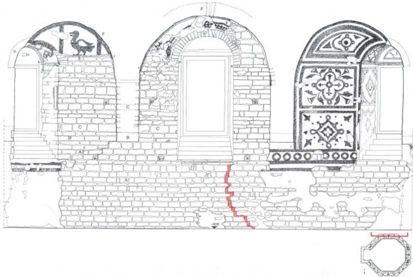
Figure 12. Detail of the outer wall of the north side of the attic; the obvious repaired crack is shown (in red) (by Giovannini 1996).
