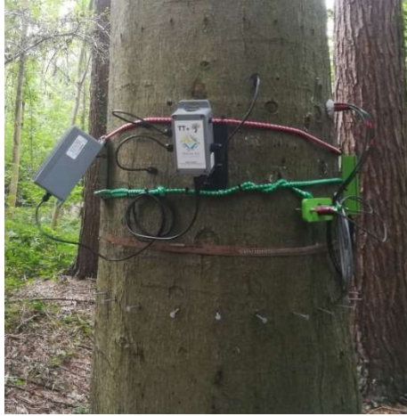
Figure 5. TT+ and TreeWatch installation on a beech tree, UGent, Belgium.
