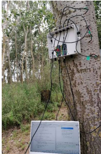
Figure 4. Installation of two pairs of TT+'s sap flow probes on P. nigra , recording high frequency data of heat dissipation, Unitus, Italy.
