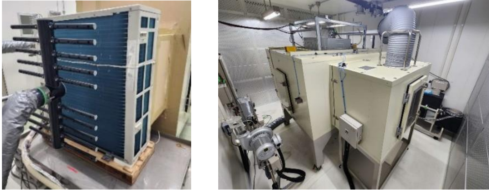
Fig. 3 Photographs of the tested system in the outdoor (left) and indoor (right) psychrometric rooms with the corresponding measuring chambers.
