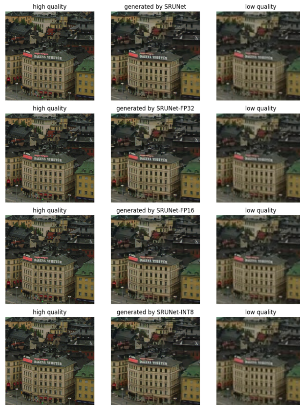
Figure 1. Qualitative results evaluating SRUNet, SRUNet-FP32, SRUNet-FP16, and SRUNet-INT8 models on a compressed and down-scaled 96 \times 96 patch of a test video frame producing a 384 \times 384 patch displayed in the middle column, along with the ground truth (left column), and the resized version using bicubic interpolation (right column).
