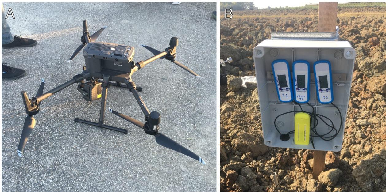
Figure 3.7. Soil temperature monitoring at the SMN site. (a) DJI Matrice 300 UAV used during the September 2022 thermal survey. (b) Gradient monitoring station installed in November 2023, comprising three XS Mini T1 dataloggers at different soil depths (~66 cm, ~20 cm, and surface) and a Mini TH sensor for air temperature and humidity measurements.
