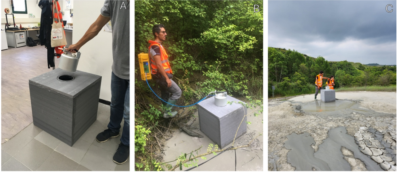
Figure 3.6. Floating extension structure for accumulation chamber measurements at Nirano. (A) Laboratory view of the high-density EPS structure designed to enlarge the chamber volume and ensure buoyancy. Field application of the modified device on bubbling mud pools at Nirano, with the accumulation chamber placed on the circular opening at the top of the structure. (B) Polla F mud Pool and (C) mud pool close to La Giunta.
