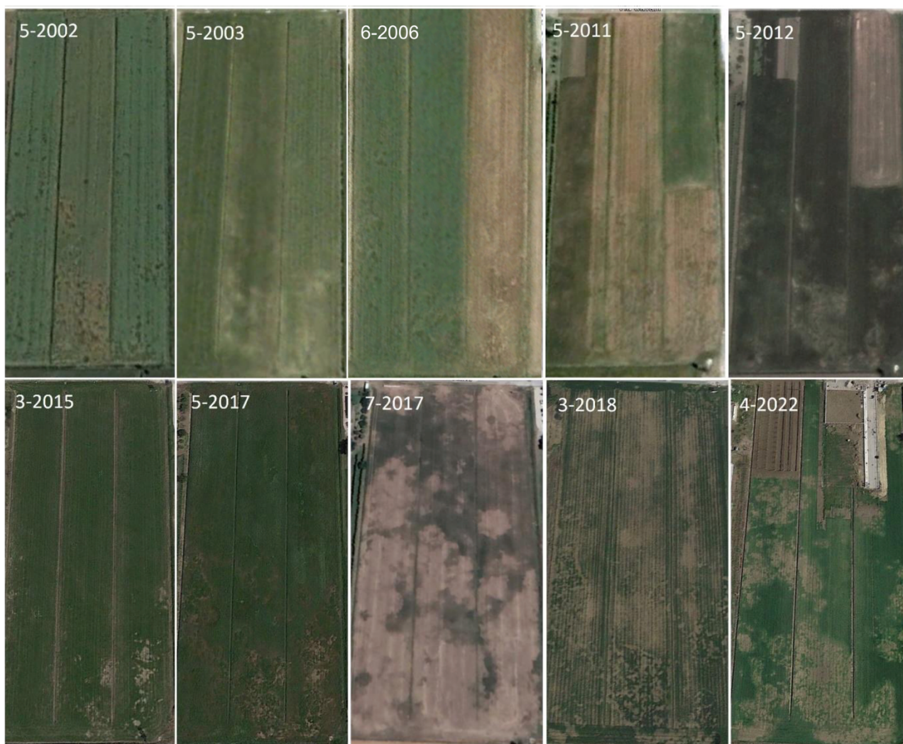
Figure 3.14. Time-stamped Google Earth Pro imagery (2002–2022) showing the recurrence of bare/sparse vegetation patches at SMN (white dates indicate month–year). These observations motivated the satellite-based RVI analysis described in the text.
