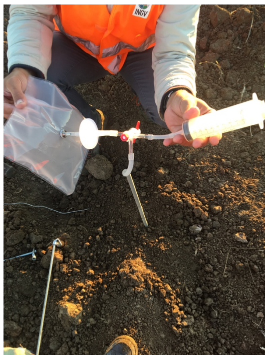
Figure 3.4. Display of the stainless-steel probe inserted into the soil and connected to the three-way valve linking the syringe and sampling bags at the SMN site.
