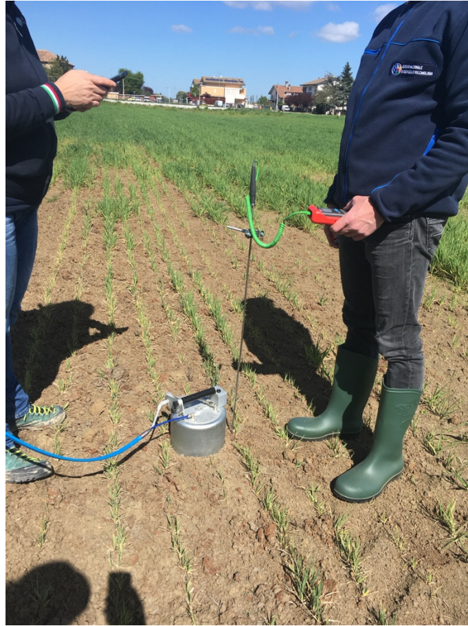
Figure 3.5. Example of soil gas flux measurement with the accumulation chamber at SMN during field surveys. The photo (April 2023) illustrates chamber deployment on cultivated soil under typical site conditions of sparse vegetation.
