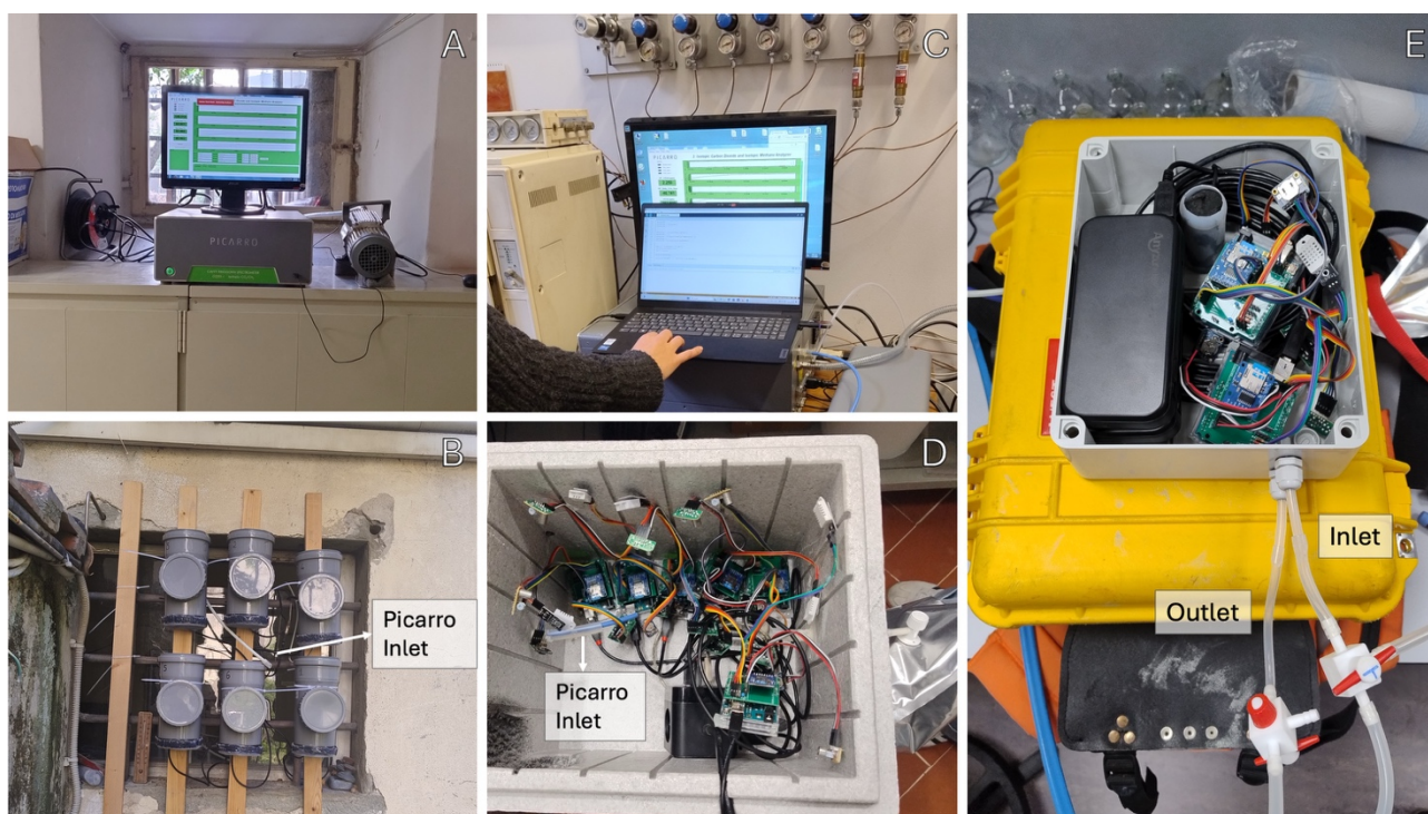
Figure 3.11. Experimental calibration setups of the low-cost monitoring stations. (A–B) Phase I: collocation of all stations with a Picarro G2201-i analyser, used as reference instrument, under ambient atmospheric CH 4 concentrations. (C–D) Phase II: controlled enclosure tests, where the stations were exposed to CH 4 -enriched gas sampled from the Renazzo well, allowing calibration across intermediate concentrations under regulated temperature and humidity conditions. (E) Phase III: portable setup for exposure to high CH 4 concentrations, using an accumulation chamber coupled with a TLD analyser to extend the calibration range up to ~16,000 ppm.
