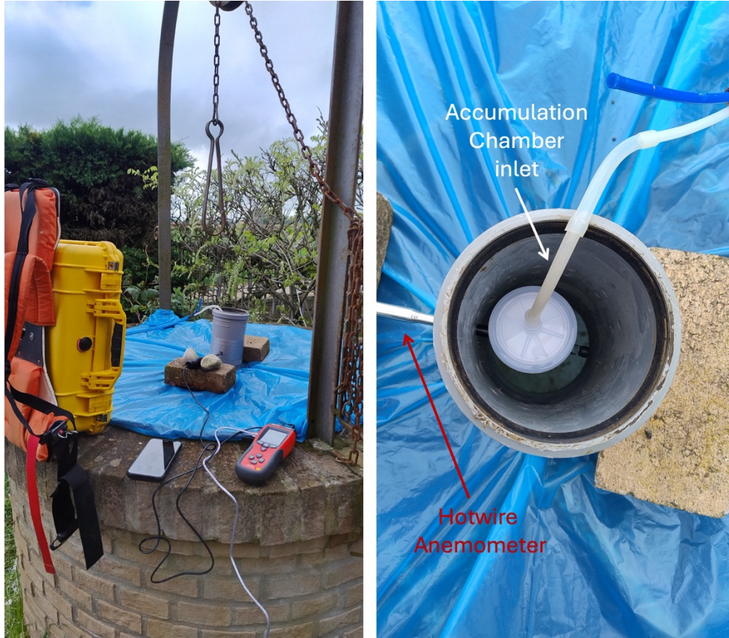
Figure 3.9. Reduced-aperture configuration (M2) applied on 15 April 2025 showing tarp constraining the emission to a central orifice ( A_r ) while the a hot-wire probe RS-8880 measured axial velocity co-located with the chamber inlet of WS-LI820 for concentration, enabling co-registered velocity–concentration flux estimates.
