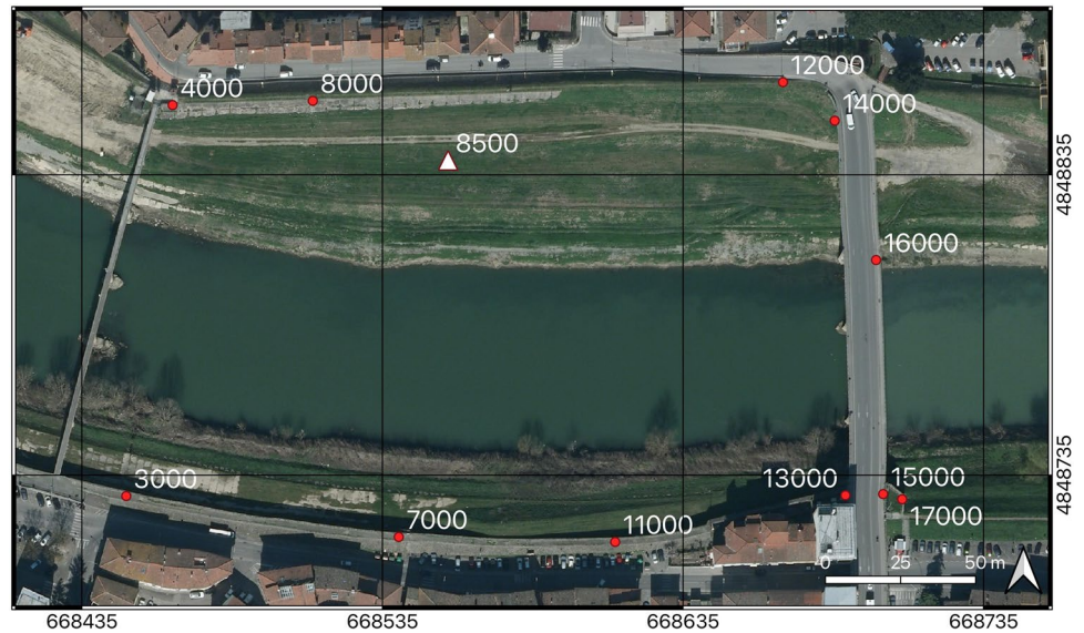
Fig. 11 Orthophoto with control network's vertexes
