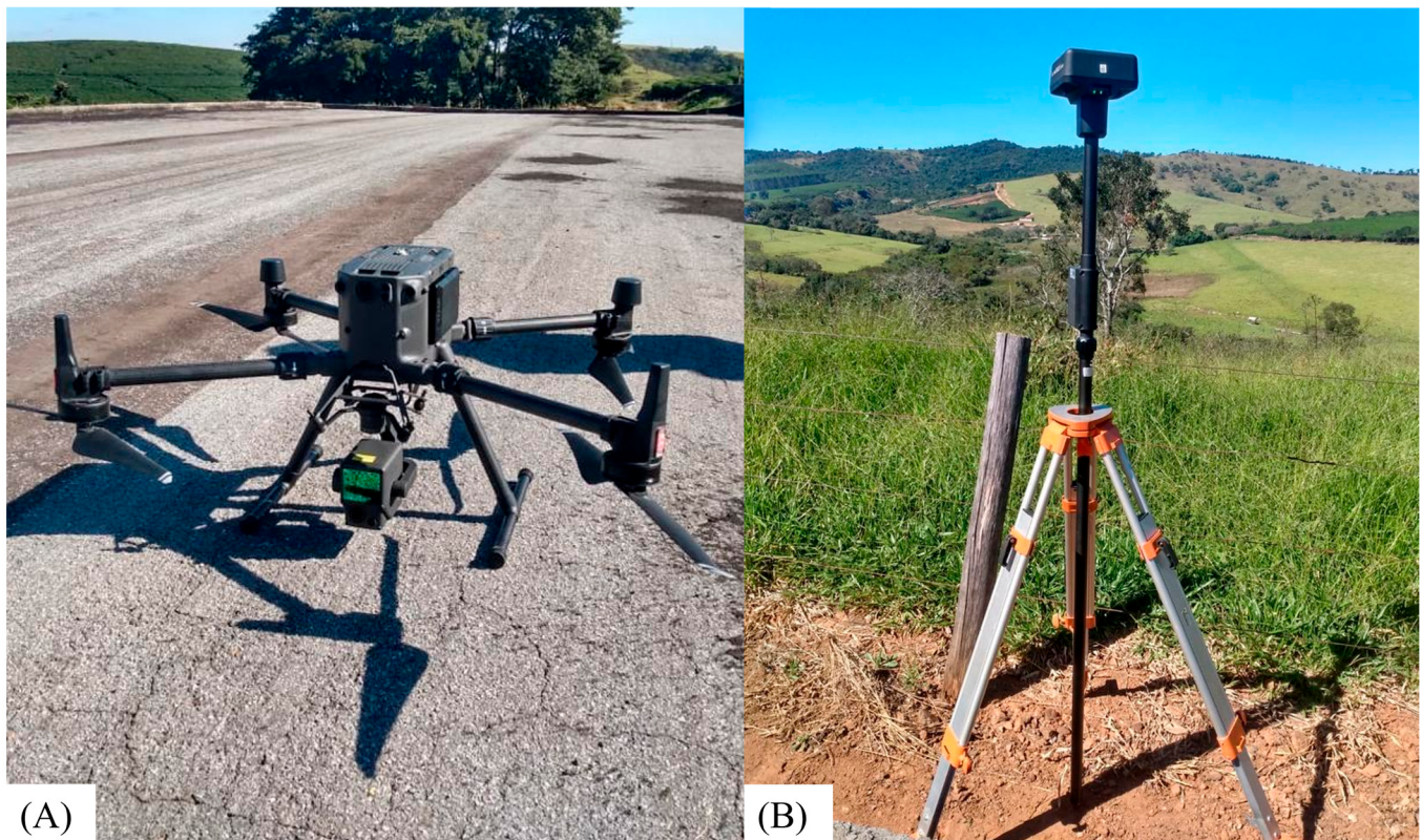
Figure 2. (A) Matrix 300 RTK coupled with Zenmuse L1; (B) DRTK-2 base fixed to the ground.
