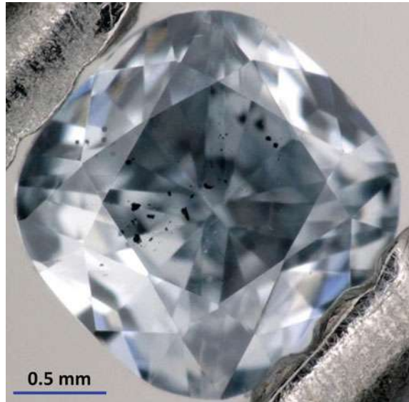
Fig. 10.6 Ferropericlasite inclusions (50–100 \mu\text{m} black minerals) in blue, super-deep diamonds (Smith et al. 2018). Photo by Evan Smith, GIA
