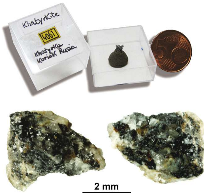
Fig. 1.4 Different views of the original museum sample belonging to the Natural History Museum of the University of Florence, Italy (catalogue number 46407/G). The lighter-coloured material on the exterior contains a mixture of spinel, clinopyroxene and olivine. The dark material mostly consists of khatyrkite ( \text{CuAl}_2 ) and cupalite ( \text{CuAl} ), but also includes granules of icosahedrite with composition \text{Al}_{63}\text{Cu}_{24}\text{Fe}_{13}
