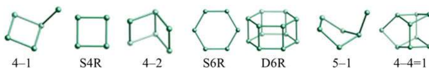
Fig. 12.7 A selection of 7 out of 23 Secondary Building Units (SBUs) from IZA-SC database ( https://europe.iza-structure.org/IZA-SC/SBUList.html )
