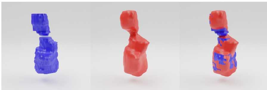
Figure 4.10: Neuron Grouping Artifacts: objects that are too close together can sometimes be mistaken for single entities. From left to right we have the ground truth annotations, the network’s prediction and an overlap of the two.
