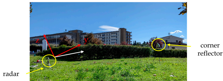
Figure 7. Measurement setup for the tests in controlled scenario with a single corner reflector. As the radar is tilted up, the white arrow evidence the direction between radar and corner reflector.
