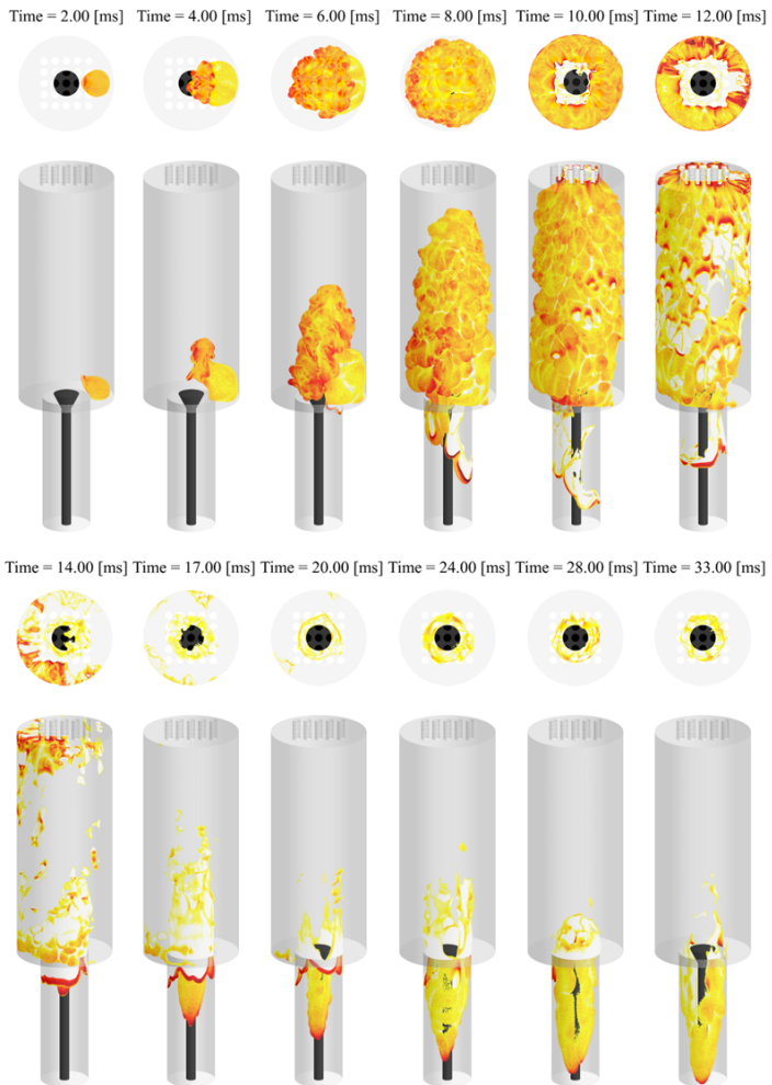
Figure 4.29: 3D flame visualization using an isosurface of HRR ( 10^8 W.m^{-3} ) colored by temperature for FB1Sr.
