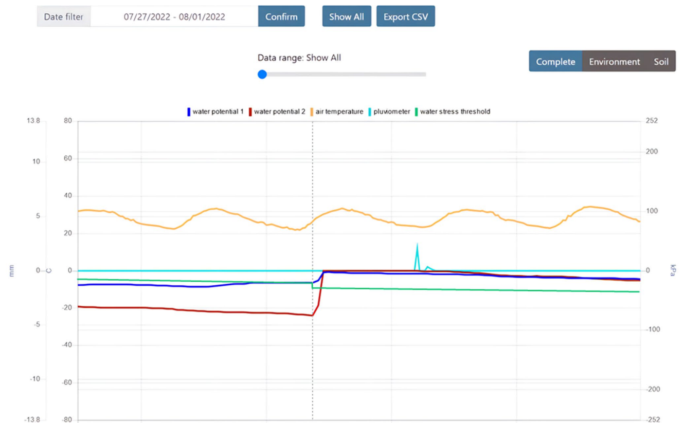
Fig. 1 Environmental and soil parameters monitored during the growing: datalogger with soil water sensors at two different depths (15 cm and 30 cm) Soil water potential - SWP1 (blue), Soil Water potential -
