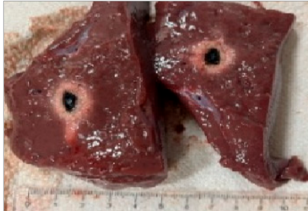
Figure 2. Single Fiber N°1 (5W@1800J). L = [19.3 \pm 1.0] mm and W = [12.5 \pm 0.6] mm (5W@1800J, 4 samples tested).
