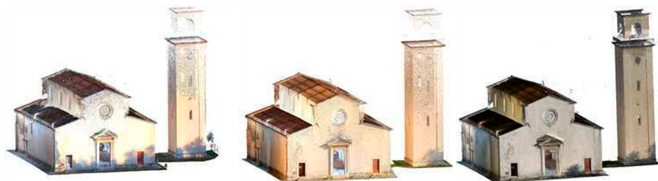
Figure 8. Vallecchia Church: data acquired respectively with the X70GO, VLX 3 and Lixel L2 Pro.
