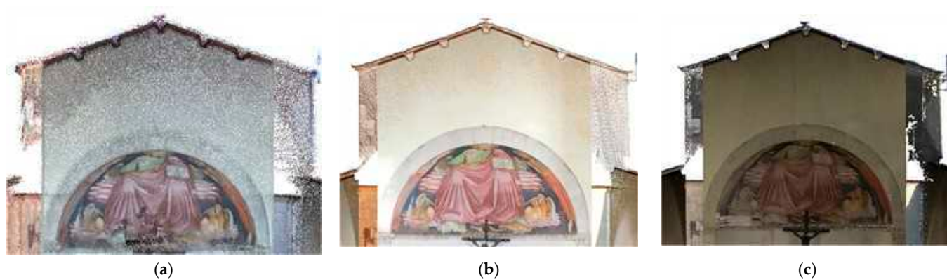
Figure 16. Vallecchia Church: point cloud of the tympanum of the triumphal arch: (a) X70GO (834,096 points), (b) VLX 3 (3,141,418 points), and (c) Lixel L2 Pro (6,747,285 points).
