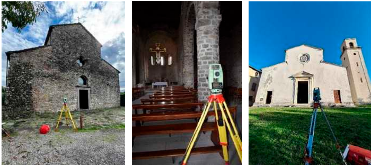
Figure 4. Total station surveying: Sorano Church (left and centre) and Vallecchia Church (right).
