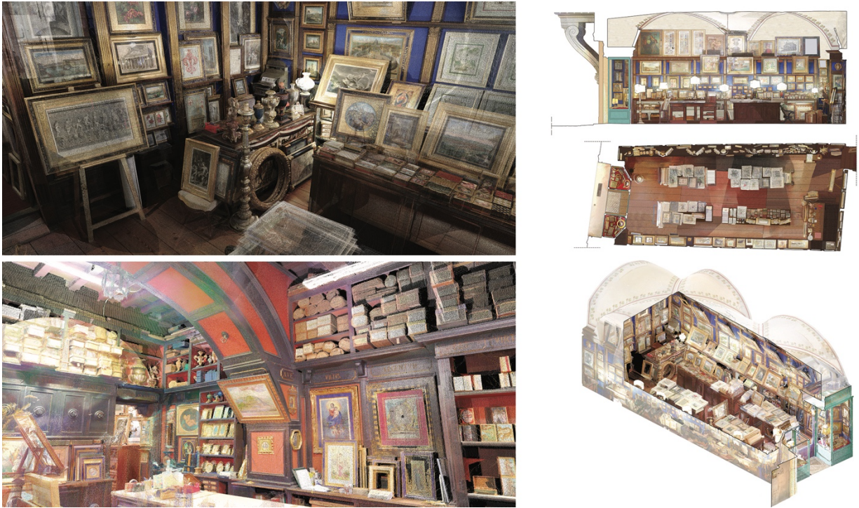
Fig. 4 Perspective images of the colored point-cloud and technical drawings of the Baccani shop for frames, prints and chandeliers in Borgo Ognissanti, Firenze.
