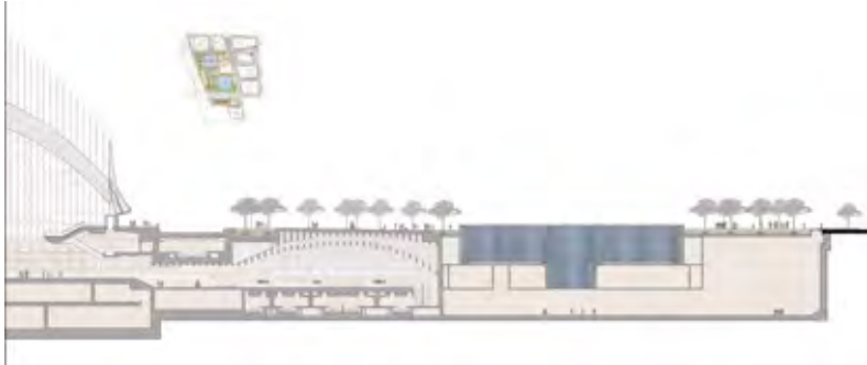
Figure 48. Cross section on Calatrava's station and on the North pool (section E-W). Credit: 9/11 M&M.
