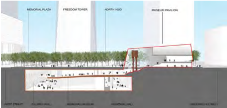
Figure 59. Cross section on the Hall and on the ramp (E-W). Credit: The N9/11 M&M and Davis Brody Bond Architects.
