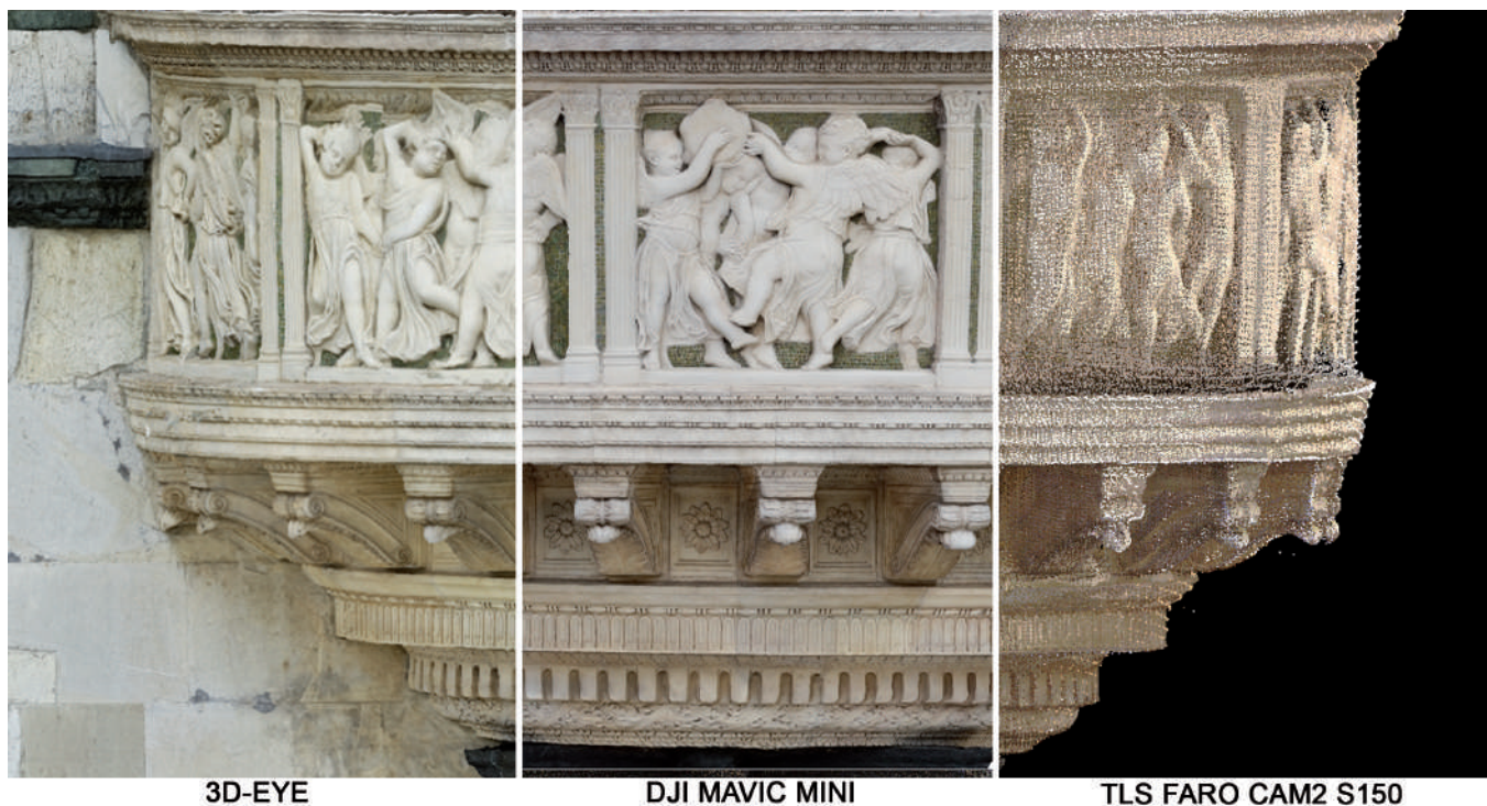
Figure 10. Composition obtained by merging three-dimensional databases coming from different instruments.
