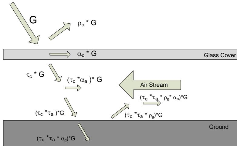
Fig. 2. Schematic of solar radiation transfer process.
