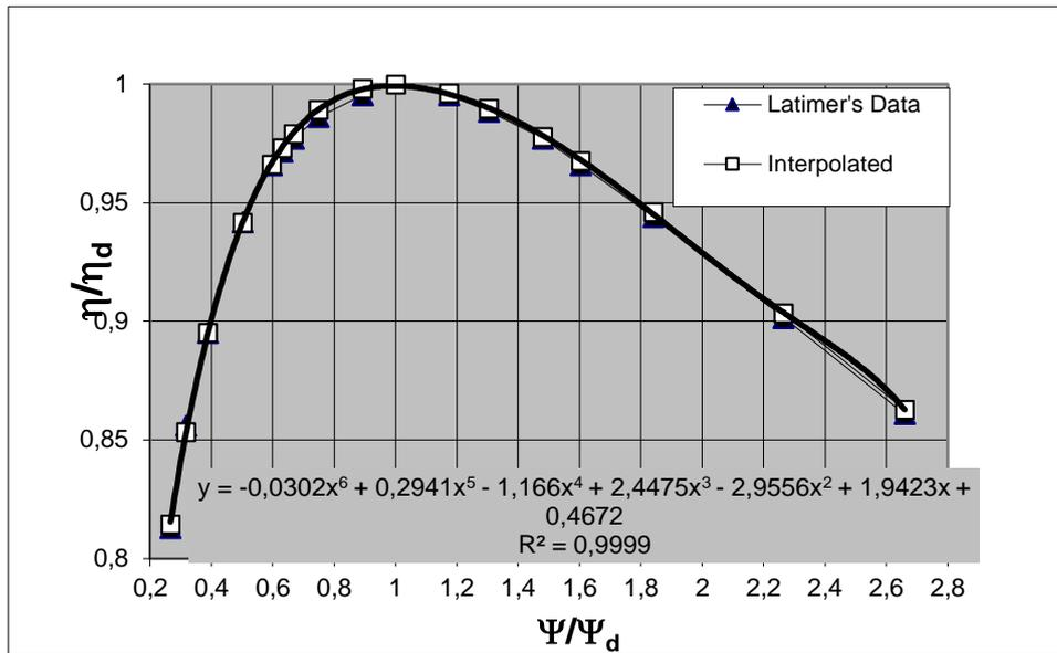
Fig. 8. Off-design Efficiency correlation (adapted from [24])
