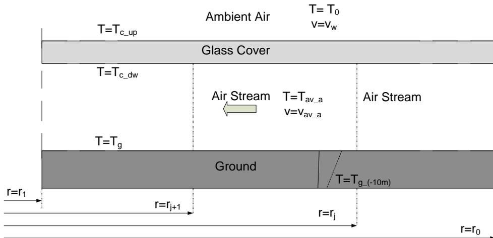
Fig. 3. General schematic of solar collector heat transfer.
