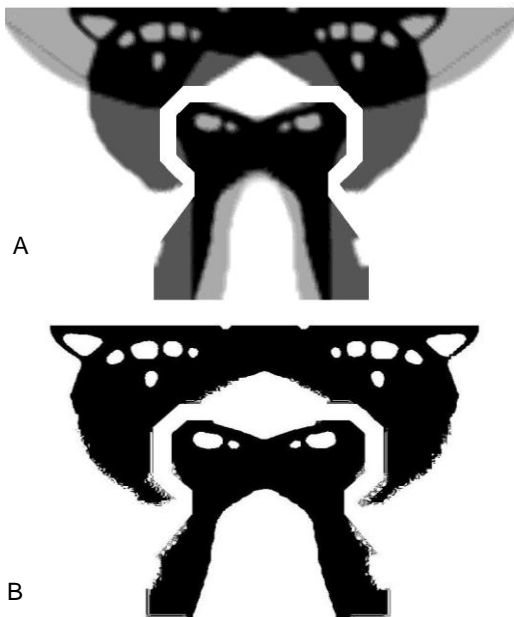
Figure 14: Above (A): hybrid solution obtained through the application of formula (1) to topologies “A” and “B” of figure 12. Below (B): resulting topology after applying a threshold equal to 0.85 to the density distribution in order to have a total mass of 16.5 kg/m.
