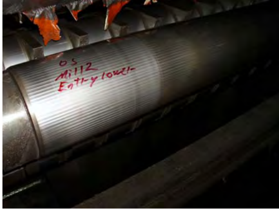
Fig. 2. Chatter marks on the roll
